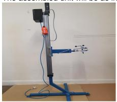
e) Secure the assembled unit to the floor by fitting a bolt of sufficient length into 3 of the outer holes in the base frame. Fit the M12 x 60 levelling foot into the 4<sup>th</sup> hole and secure with the locking nut. Tighten the 3 bolts securely into the drilled holes in the floor and adjust the levelling foot to ensure the unit is level and stable.
